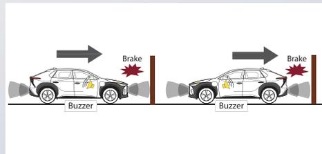
Detection covers a wide area surrounding the vehicle, helping to avoid minor collisions and reduce damages.
